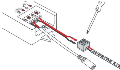
**5.** Use #1 Phillips to loosen the 4 terminal screws on 8MM-EZ Connector. Peel 1/2" of the adhesive protector from back of LED tape light, insert into connector, evenly tighten screws. Insert wires from Receiver into terminals, Red wire to (+) side of tape, Black wire to (-) side of tape; tighten screws.
