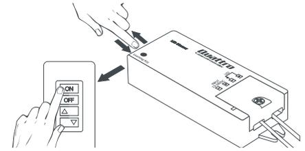
**3.** Quickly press and release the Learning button and, within 5 seconds, press and release one of the 1-Zone buttons on the Controller. When lights blink once, Controller and Receiver are paired.
