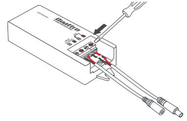
**3.** Use a flat blade screwdriver to loosen terminals for the Male Plug and remove.
