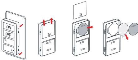
**1.** Remove Controller from back plate, slide battery compartment open, remove battery, and discard clear plastic tab. Reinsert battery, replace cover.
