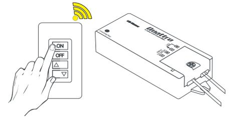
**6.** Turn on 120V AC to Power Supply and pair Receiver to Controller.
