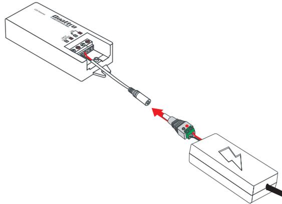
Wire a Male Barrel Connector to the output wires on the low voltage side Power Supply, Red wire to (V+), Black wire to (V-). Plug into Female Plug Connector on the Receiver.
