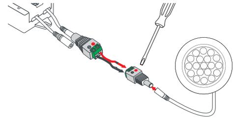
**3.** Insert Male Barrel Connector to Female Plug on Puck Light. Use Flat blade screwdriver to loosen screws on Male Barrel Connector. Insert wires, Red wire to (+), Black wire to (-), and tighten screws.
