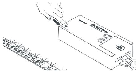
**2.** Clear the receiver by pressing and holding the Learning button until the lights blink twice
