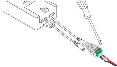
**2.** Insert Male Plug on Receiver into Female Barrel Connector. Use Flat blade screwdriver to loosen screws on Female Barrel Connector. Insert wires, Red wire to (+), Black wire to (-), and tighten screws. Insert the other end of wires into EZ-WSC Connector.
